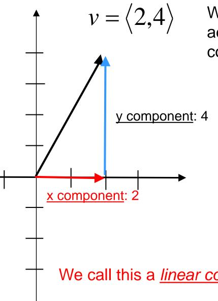
We could rewrite this as the addition of the x and y component vectors.
